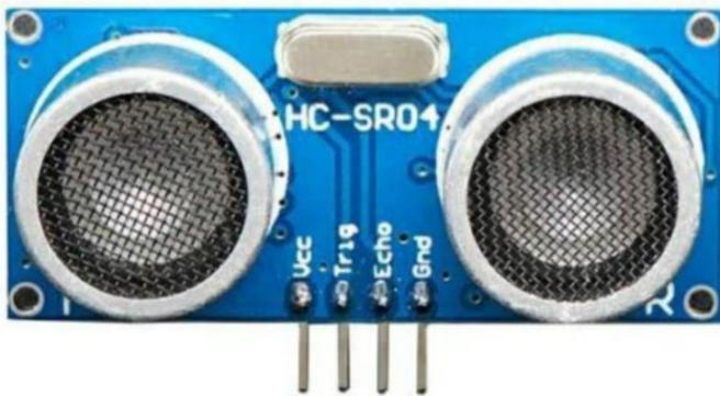
Figure 8: Ultrasonic Sensor
